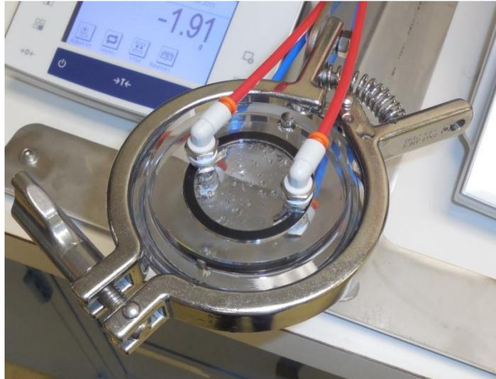
**Figure 7.3 - Circular FO cell with an effective membrane area of  $1.257 \times 10^{-3} \text{ m}^2$**
